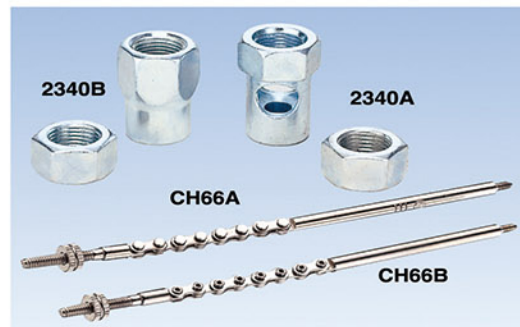
66A/66B CH66A For sturmey-archer; 3-SP hub length: 135mm CH66B For sturmey-archer; 3-SP hub. (5-SP optional) Length: 126 mm 2340A/2340B 2340A 13/32"-26T/1007, 1008: Axle nuts for sturmey-Archer 3-SP hub U.C.P. finished; 2340B 13/32"-26T/1009, 1010 Axle nuts Torpedo F & S 3-S Phub.; U.C.P. finished
